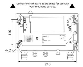
Drill holes to the surface according to holes spacing. Mount Subdrive via mounting holes to the surface.
