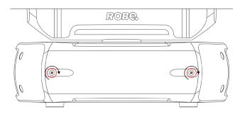
Fasten the additional cover to the base of fixture with two "quarter-turn" locks.
