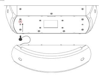
Secure the display cover by fastening the "quarter-turn" lock with safety wire attached into the base of fixture, as illustrated.
