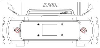
Loosen "quarter-turn" lock on each side of display frame.
