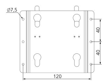
Prepare 6 holes into the ceiling according to the spacing of the mounting kit holes and dimension illustrated above.
