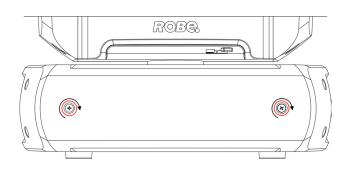
Fasten the display cover to the base of fixture with two "quarter-turn" locks.w
