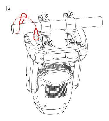
Secure the fixture to the pole via safety wire with carabiner on each end. One carabiner installed inside the base of fixture and other around the safety wire to create a loop around the pole. As illustrated on the picture.
