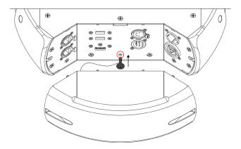
Secure the additional cover by fastening the "quarter-turn" lock with safety wire attached into the base of fixture, as illustrated.
