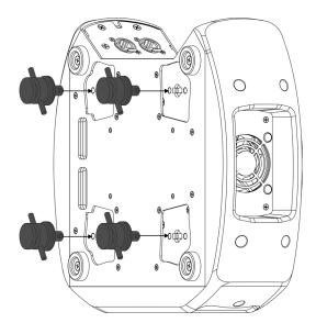
Insert 4 CAMLOCs into the 4 locks from the bellow of fixture's base.
