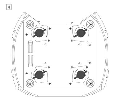
Turn the CAMLOCs clockwise (as illustrated) until it snaps into locked position.
