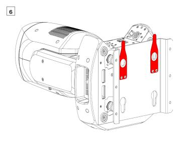
Insert the fixture with installed CAMLOCs into the mounting kit, by pushing the safety lock and sliding into locked position. CAMLOCs must be secured by snapping the safety lock into position.
