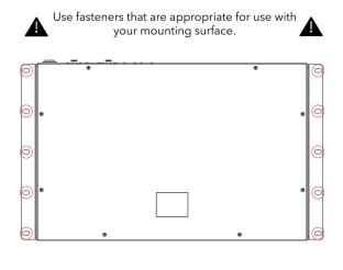
Drill holes to the surface according to holes spacing. Mount ArcPower Unit Pixel via mounting holes on the surface.
