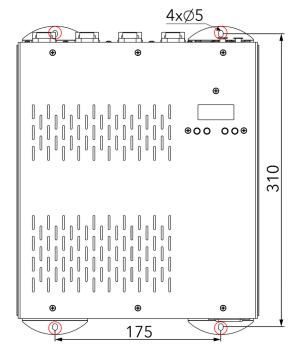
Fasten the ArcPixel Power to surface via four mounting holes and four screws.
